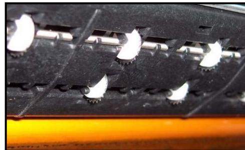
5. Immediately after wetting the nozzles surface, GENTLY close the clamshell. **CAUTION:** To prevent damage, hold onto, then lift and release both latches when closing. If you force it closed without holding the latches open, you will eventually damage the latches and clamshell switch (door switch).
