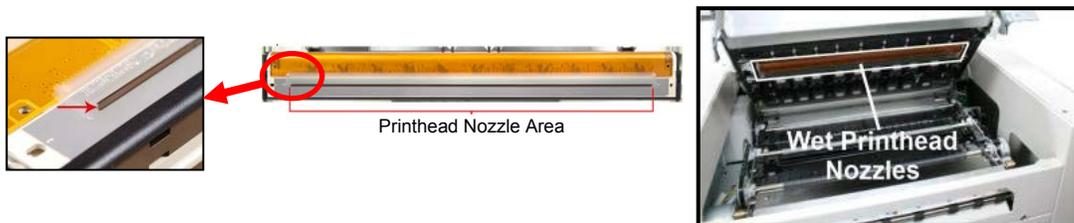
**WARNING:** Be careful not to damage the “star rollers” when wiping the printhead. These rollers are designed so they can roll across a wet image, without damaging the image. If the rollers are bent, they will not turn free; causing media feed issues (jamming) and possible damage to the image or media.
