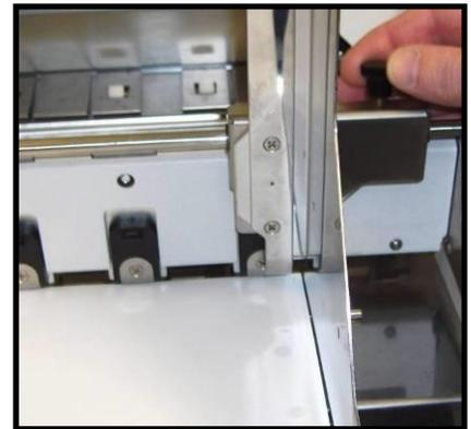
**Tip:** If the right edge of the media is damaged, during transport through the print engine; try repositioning both of the media side guides so the Adjustable Media Side Guide is no less than 1/8" away from the side frame.
