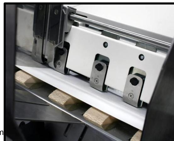
5. Loosen the separator locking screw and allow the separator to settle onto the media. Then tighten the locking screw. Repeat for each sheet separator.
