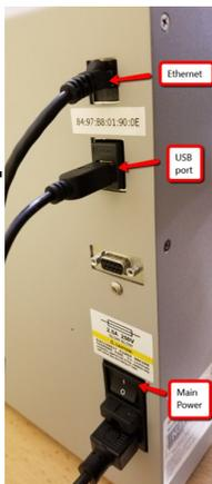
➡ **Power** - Four 110v/115v outlets total of 10 amps power will need to be available within 6ft of the unit.
