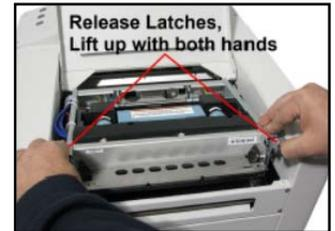
8. Slowly close the Printhead Latch until it locks. It will be resistant, but apply consistent pressure and the ink couplings will ease into the ink ports on the printhead. Once latch is closed, the printer will automatically start running a “printhead priming routine”. See “What to Expect” below.
